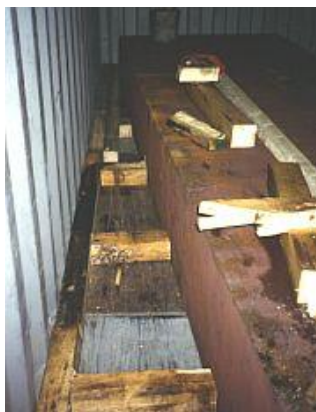
Figure 7.45 Transverse blocking of steel slab
