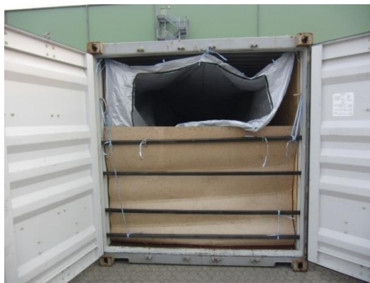
Figure 7.54 CTU with liner bag for accommodating a sensitive bulk cargo
