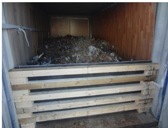
Figure 7.55 CTU with wall liners and door barrier loaded with scrap
