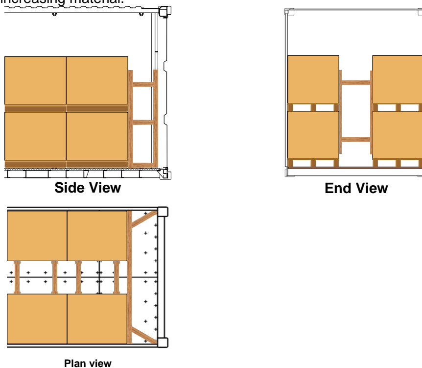
Figure 7.32 Blocking in a strong boundary CTU
